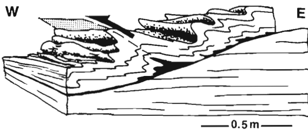
Fig. 4. Illustration of folds developed above a weak slip zone in gneissic tectonites in the basement below the Bergsdalen Nappes (near Straume). The reverse slip component caused by the folding is indicated. Based on field sketch and photograph.
